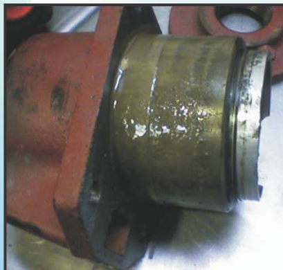
The RM410 Piston Air Motor showing signs of water contamination
