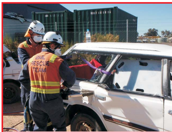
An Endless Sling secures the door & the pillar ensuring that the door will not spring open
