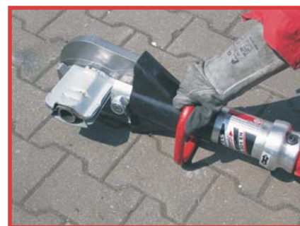
Lukas Cutters cutting through a boron re-enforced pillar.
