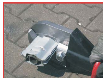
Note that the pillar is sitting directly against the Notch.
