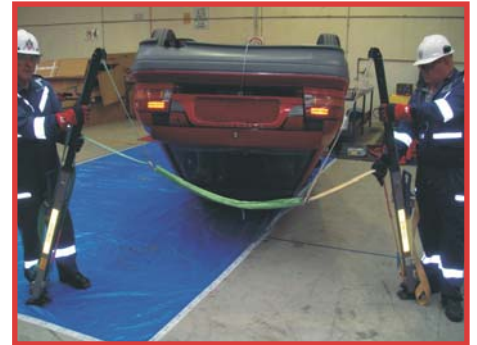
Above: Rated Endless Sling placed between the Stabfast hooks before positioning against the vehicle.
