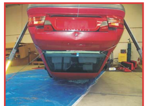
After positioning & ratcheting, the rear window offers a clear space for access & casualty removal.
