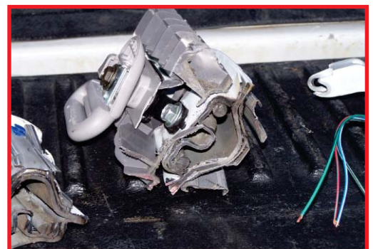
Subaru B-Pillar strengthened by two Reinforcement Bars
