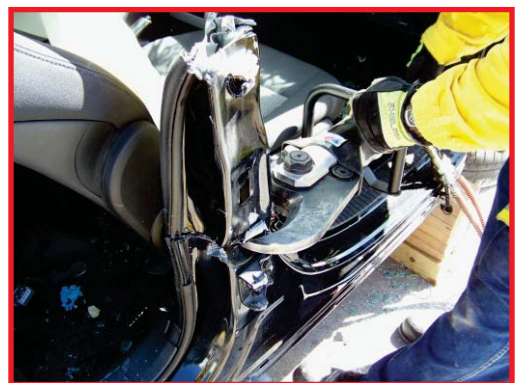
Subaru B-Pillar strengthened by two Reinforcement Bars
