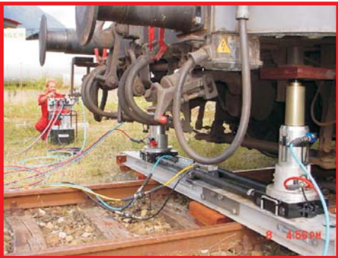
Lukas Duo Re-Railing System consisting of Pump & Controller, Lifting Jacks, Traversing Bridge and Roller Carriages
