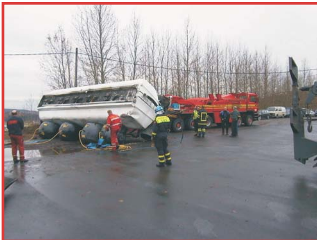
Vetter Low Pressure Airbags being used to right an overturned vehicle
