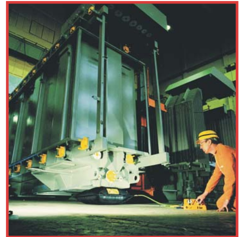
Vetter Airbag being used in a Lifting Application
