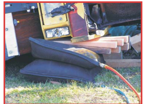
What not to do! Never place objects between the bag & the load as they have the potential to be ejected
