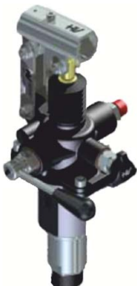
Two Speed Hand Pump with release hand knob and exclusion lever for first speed, for use with Single Acting Cylinders
