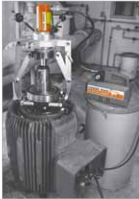
SGH153CR with a bearing pulling attachment was used to take a bearing off a utilities well pump motor.
